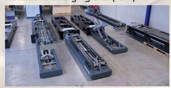
In 2006/2007, DFW Europe launched a unique and unrivaled Automatic Charging Bier (AIM). The AIM is installed under the cremator and is only visible when the coffin is charged. The AIM provides an ergonomic solution for the insertion of coffins weighing up to 250kg into cremators operating at over 650°C.
